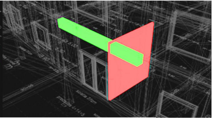
CLASH DETECTION: ARCHITECTURAL- STRUCTURAL-MEP
